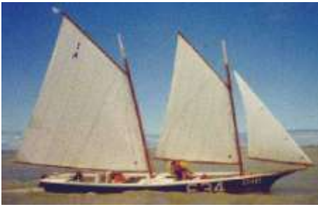
A Phil Bolger "Light Schooner", a 24' long centerboarder and blazing fast, was recently donated to MHA.
