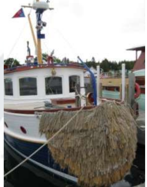
It's not a beard, it's a "bow pudding!" on the tug Restless , fresh from her win at the The Great Tugboat Races in Sault Ste Marie.
